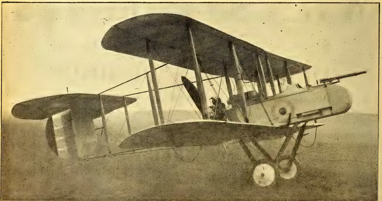
THE VICKERS "GUN-BUS."—The first successful aeroplane designed specifically for fighting. During 1915 and 1916 these machines, with 100-h.p. Monosoupape Gnome engines, did excellent work in France, and continued to do so long after they should have been considered out of date by any thoroughly organised supply department.
